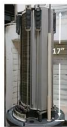
SOFC Stack 7 kW DC Power Generation 36 kW DC / 25 kg H 2 /day electrolysis 350 cells, 17" height
